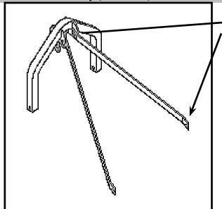
Attach A-Frame Braces to A-Frame and Deck with hardware provided.
