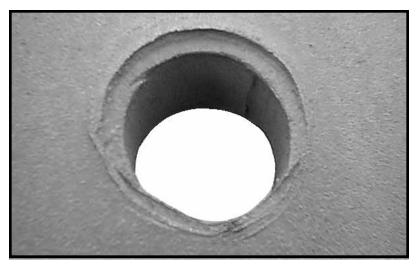
the blade to jam so that it can no longer pivot on the blade bolt. A jammed blade will break either from fatigue or from catastrophic occurrence and will allow the blade to be ejected. A blade carrier damaged in this manner must be taken out of service immediately. Repair the blade carrier (contact Brown Mfg. Corp. for instructions) and replace the blades and blade bolts before returning the machine to service.
