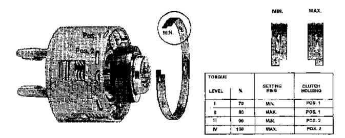
The torque setting can be modified with the aid of the setting ring and two alternative location slots in the clutch housing.
