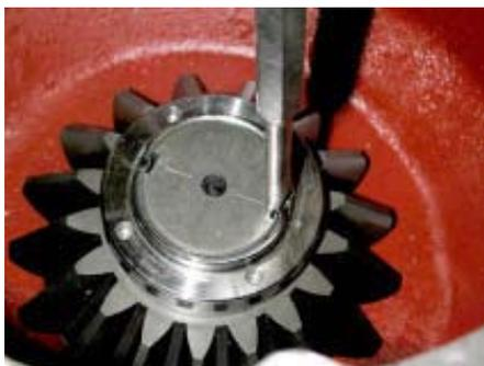
7. Place an appropriate spanner socket on the lock nut. Be sure the pins are completely engaged.
