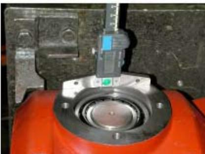
21. Measure the gap between the housing and the race of the bearing. The thickness of shims to be used is given by the difference between the two measurements, minus 0.1 mm (0.004")
