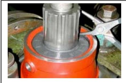
1. Remove the cotter pin (T5-052), M42x3 nut (T5-054A), output seal guard (T5-048), and the output oil seal (T5-065) from the output shaft.
