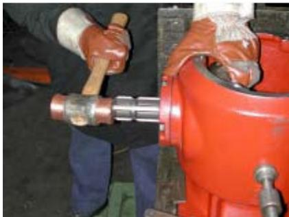
3. Remove cover opposite to the input shaft (T5-037). Remove any shims found. Remove any remaining gasket material.
