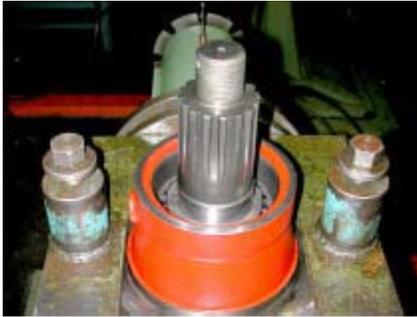
11. Remove the output shaft (T5-040), along with the inner races of the of the tapered roller bearing sets.
