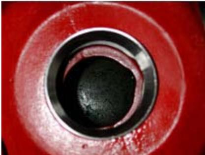
12. Remove the outer races of the tapered roller bearing sets from the casting.
