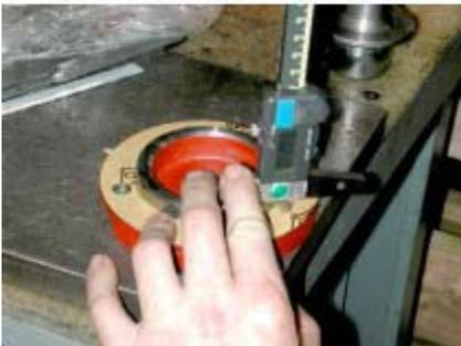
20. Place the gasket on the other cover (T5-047) and measure the gap between the shoulder and the gasket.
