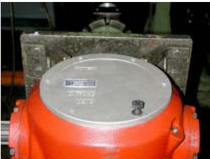
25. Apply RTV sealant to the top surface of the housing and install the top cover using the M10x20x1.5 (T5-050) bolts. Tightening torque 4.7 - 5 Kg-m (408 - 434 in-lb).
