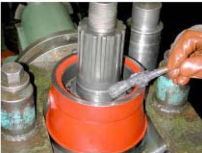
27. Lubricate the oil seal (T5-065) and the surface of the output shaft, in order to ease the installation of the oil seal.
