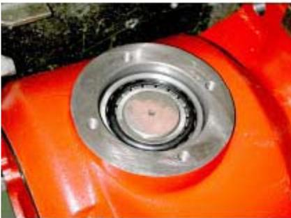
19. Install the input shaft (T5-039 1 3/4" x 6 spline or T5-039-20 1 3/4" x 20 spline), and the taper roller bearing (T5-060). Seat the shaft until all play is removed.
