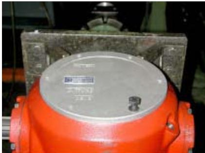
2. Remove the top cover (T5-035). Clean sealant from the surface.
