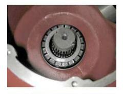
5. Install the bearing of the tapered roller bearing set (T5-061) onto the shaft.
