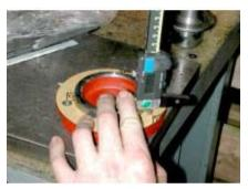
20. Place the gasket on the other cover (T5-047) and measure the gap between the shoulder and the gasket.
