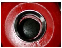
12. Remove the outer races of the tapered roller bearing sets from the casting.
