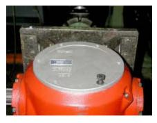
2. Remove the top cover (T5-035). Clean sealant from the surface.
