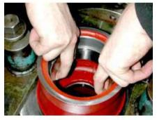
2. Check that the outer races of the tapered roller bearing sets are firmly seated in the bores.
