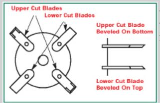
The axe-like chopping effect of the offset blade bevels give the Brown Tree Cutter unmatched cutting ability.
