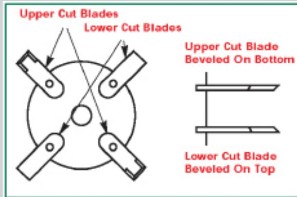
The axe-like chopping effect of the offset blade bevels give the Brown Tree Cutter unmatched cutting ability.
