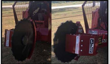
Brown Tree Saws are designed to be rugged machines that can handle selective clearing of wood lots, fence rows, food plots and ATV/bike trails. The heavy construction is tough enough to cut heavy brush and trees up to eight inches in diameter. The balanced blade keeps vibration to a minimum.
