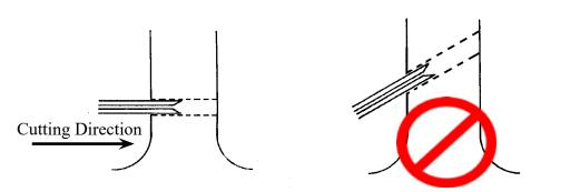
**DANGER:** Extreme pressure is being applied on the blades. This pressure can cause the blades to bend or break.
