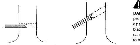
**DANGER:** Extreme pressure is being applied on the blades. This pressure can cause the blades to bend or break.
